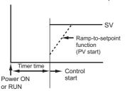
Control is performed during the timer time and stops after the timer time elapses.
