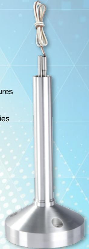
**Cast Vacuum Chamber Heaters** are designed to optimize temperature profile in a vacuum chamber. Uniform process temperature improves etch and deposition rates and uniformity.
