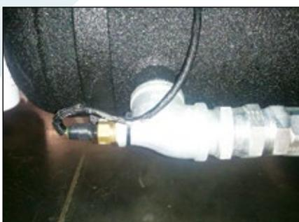
*Temperature sensor installed in power unit*
