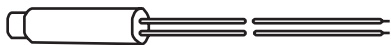
TYPE L - PTFE Lead wire 36" standard Ground lead is optional on all terminations
