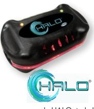
HALO<sup>®</sup> is a patent pending integrated controller that reduces thermal system complexity and cost as compared to traditional solutions. Combined in one controller are multiple sensor inputs, including process temperature, limit temperature, and current sensing that allows monitoring of multiple heaters wired in parallel. Designed to be used in remote locations that may not be easily accessible by maintenance
